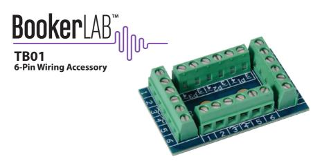
The TB01 6-Pin Wiring Accessory from BookerLAB provides easy, screw terminal connection to multiple Leslie® speakers. It provides 1:1 terminal blocks between up to three Leslies® with a separate AC power terminal for relay or other custom power distribution arrangements.
