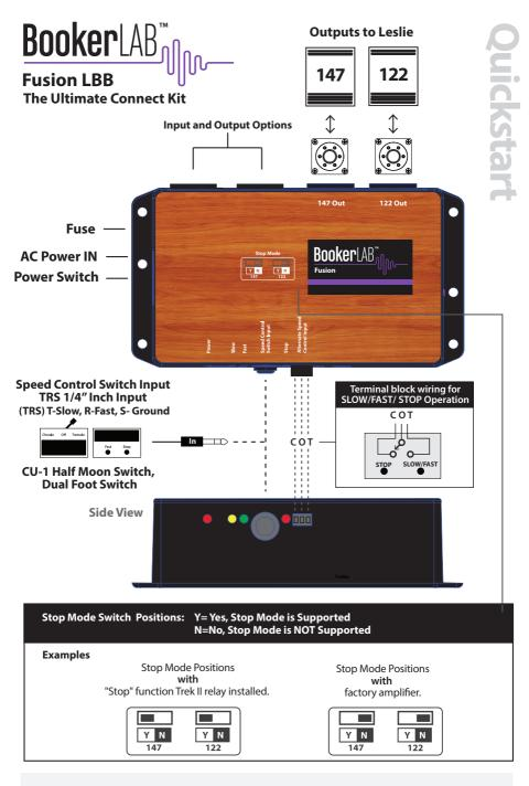
BookerLAB was created to maintain the quality of vintage musical instruments and supporting equipment, specifically the Leslie<sup>®</sup> Speaker Cabinet. BookerLAB offers a range of products for interfacing gear, conversion, motor control, and amplification. With products built solely in America, we've developed these unique systems in collaboration with music industry partners. Explore our story at www.bookerlab.com.
